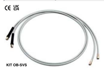
Two high pressure Kevlar stranded flexible hoses with pre-crimped fittings and bend restrictors on both ends. Recommended for use with all Ultraflex SilverSteer<sup>™</sup> and MasterDrive<sup>™</sup> helms with 1500 psi relief valves. Lenghts available: from 3m (9.8') to 9m (29.5') with 0,5m (1.6') increments.
