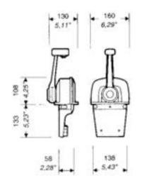
Single lever / dual action control to operate both throttle and shift. Suitable for any type of boats with inboard (B65 e B73) outboard or I/O power plants (B76 e B77, Trim version)
