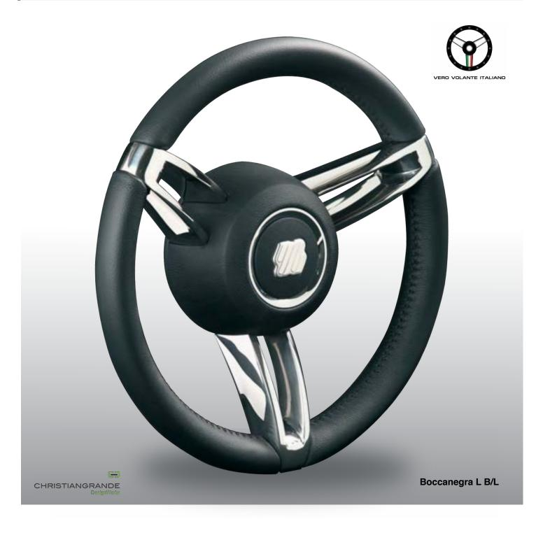
3-spoke steering wheel. 316L stainless steel polished spokes. Hand-stitching leather grip. Leather wrapped, chrome plated or painted cover. Leather wrapped or painted center cap.
