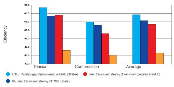
Test configuration 3 bends at 90°; 1000N load
