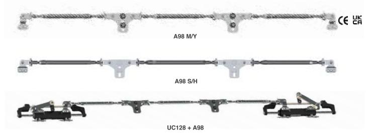
Suitable for applications with quad outboard engine and dual cylinder UC128-OBF or UC130-SVS • Also available in semi-assembled bars and brackets
