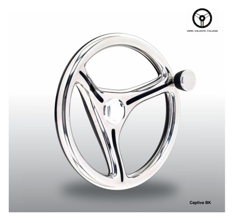
3-spoke steering wheel, available with incorporated knob or without knob. Polished 316L stainless steel and black TPU spokes with black methacrylate inserts. Polished 316L stainless steel front grip, black TPU rear grip. Polished stainless steel center nut (available as spare part). Captiva B is compatible with Knob SK 25458S as retrofit.
