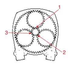
Ultraflex mechanical steering helms T71FC, T73NRFC, T91, T93ZT as well as dual cable versions and tilt wheel versions use a **Planetary Gear Design**.
