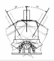
X72 43140K Tilt mechanism for hydraulic front mount steering systems
