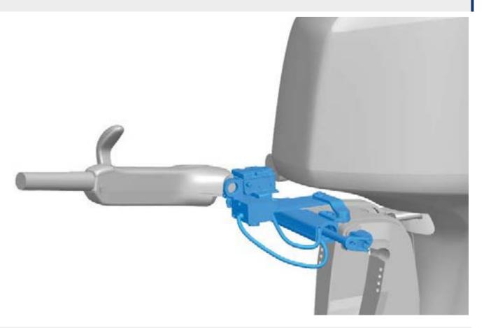
ZTF - Zero torque feedback tiller steering systems
