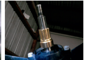
Fig. 8 The forward thrust washer MUST be installed first. Failure to install a forward thrust washer will cause gearcase damage and potential injury.
